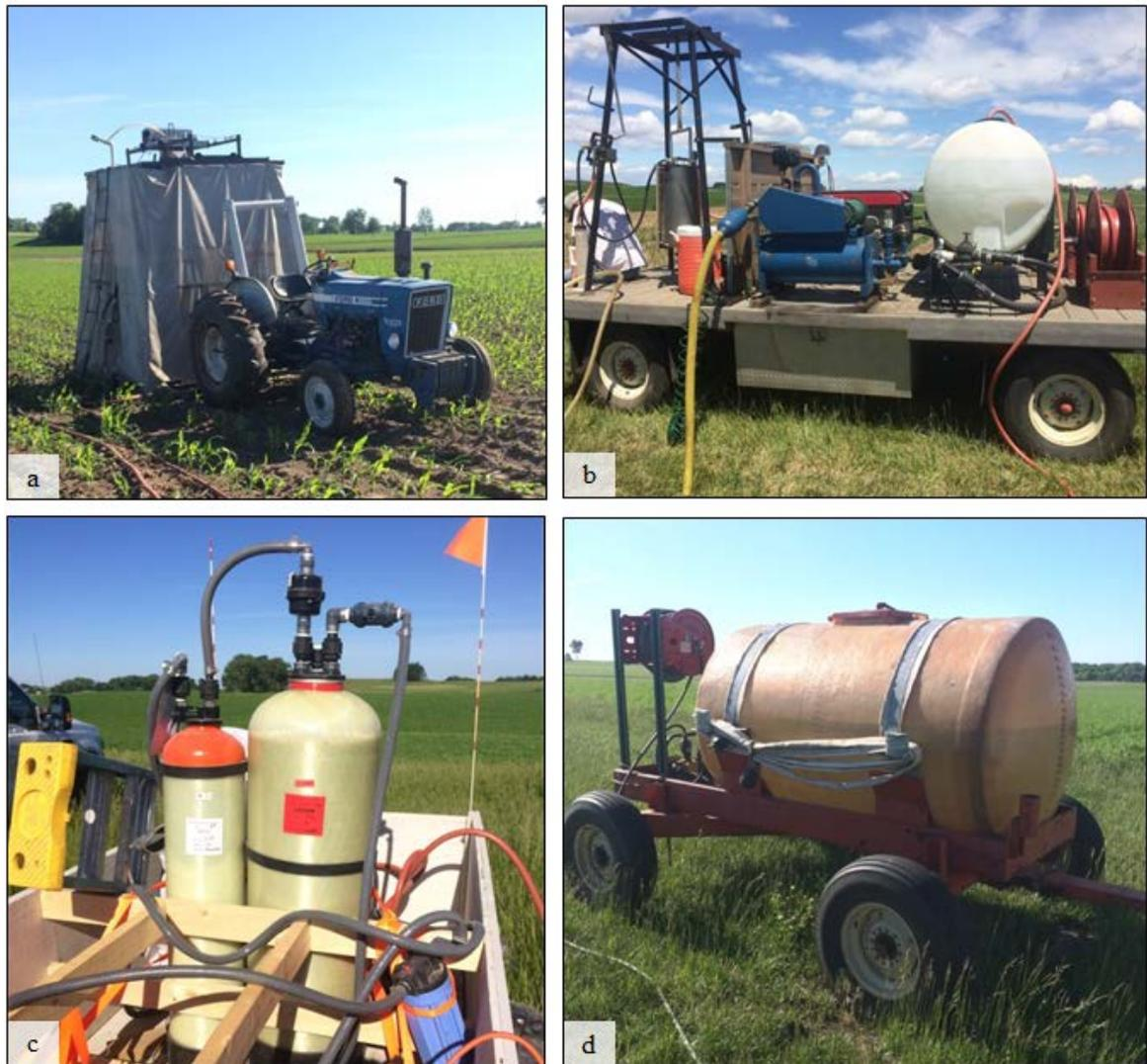
Figure 1. Rainfall simulator components consisted of (a) a water nozzle tower with tarp attached to a tractor, (b) a main wagon that housed the controls, a water tank for applying water to the nozzle, and a stainless steel collection tank to collect runoff with a vacuum hose, (c) a water deionizer system, and (d) a nurse tank water wagon that fed the tank in the main wagon through the deionizer system.
